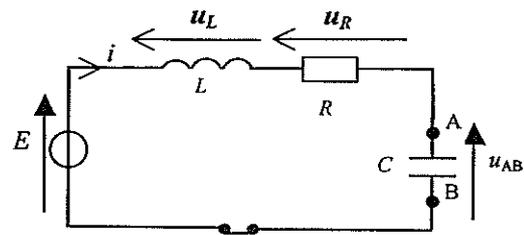
$$E = 9,0 \text{ V} \quad L = 0,10 \text{ H} \quad C = 0,10 \text{ } \mu\text{F}$$
