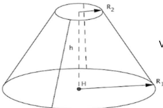
$$V = \frac{\pi \cdot h}{3} (R_1^2 + R_2^2 + R_1 \cdot R_2)$$
